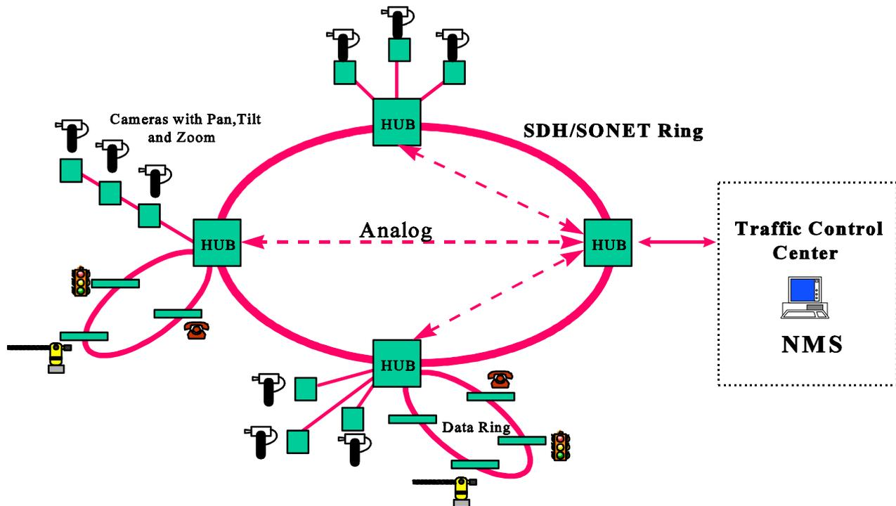
In this case, wavelength division multiplexing (WDM) allows an analog network to be overlaid onto the digital SDH/SONET ring network, thereby protecting investments incurred to date for analog equipment. This hybrid approach allows the analog and digital networks to become fully integrated such that the incoming video, voice and data signals can be *selectively* routed onto the SDH/SONET payload where applicable under the control of network management facilities.
