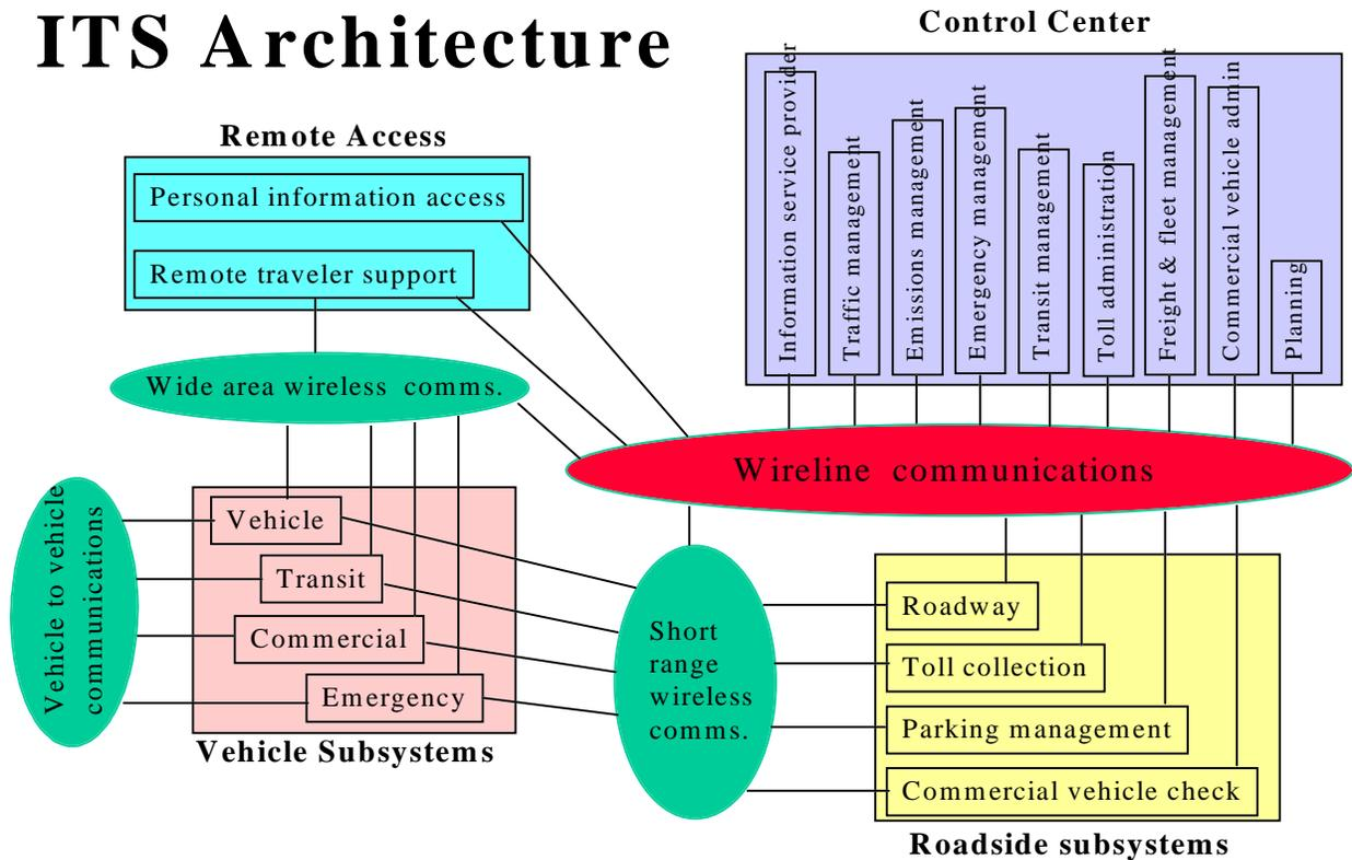
The model clearly shows four major subsystems, with the Control Center Subsystem, Roadside Subsystem, Remote Access Subsystem and Vehicle Subsystem all interconnected by a variety of telecommunications subsystems. By far the most complex of these is the so called “wireline communication networks.” This is more commonly referred to as a wide area network or WAN.
