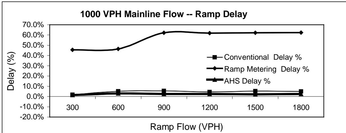
Figure 16. Ramp Delay with 1000 VPH Mainline Flow
