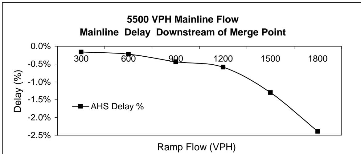
Figure 15. Mainline Delay Downstream of Merge Point with 5500 VPH Mainline Flow
