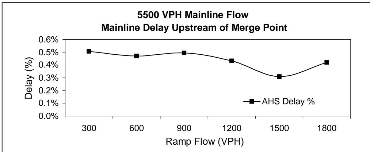
Figure 12. Mainline Delay Upstream of Merge Point with 5500 VPH Mainline Flow
