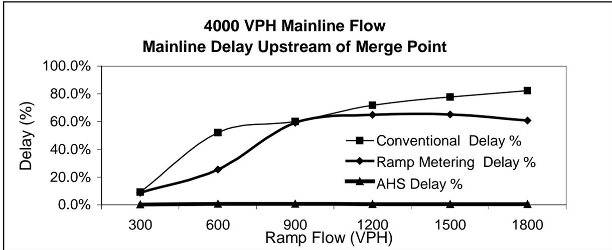
Figure 11. Mainline Delay Upstream of Merge Point with 4000 VPH Mainline Flow
