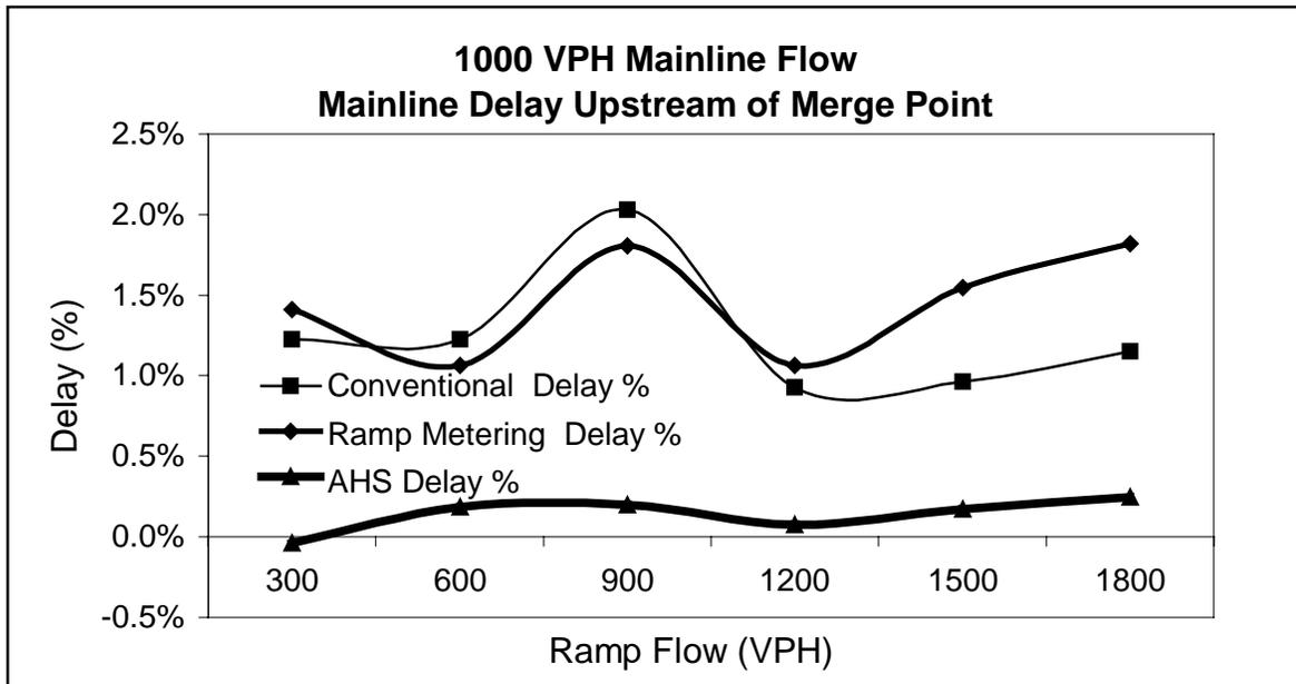
Figure 10. Mainline Delay Upstream of Merge Point with 1000 VPH Mainline Flow
