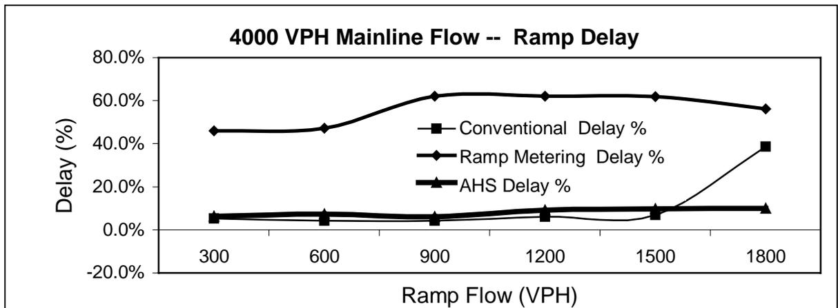
Figure 17. Ramp Delay with 4000 VPH Mainline Flow
