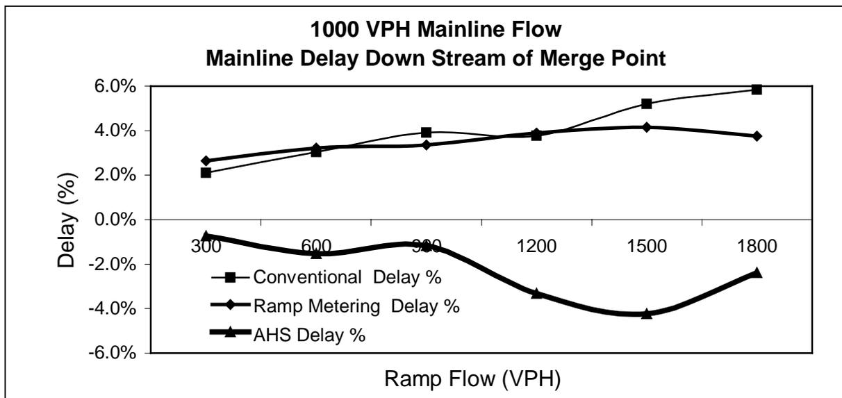
Figure 13. Mainline Delay Downstream of Merge Point with 1000 VPH Mainline Flow
