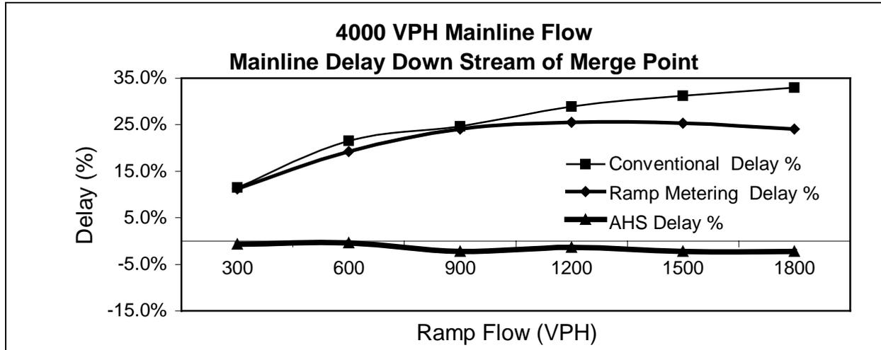
Figure 14. Mainline Delay Downstream of Merge Point 4000 VPH Mainline Flow
